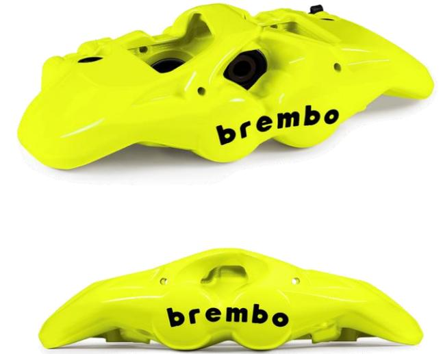
4-piston monobloc for front and rear axle applications, suitable for rotors up to 380mm x 30mm (14.96" x 1.2").
